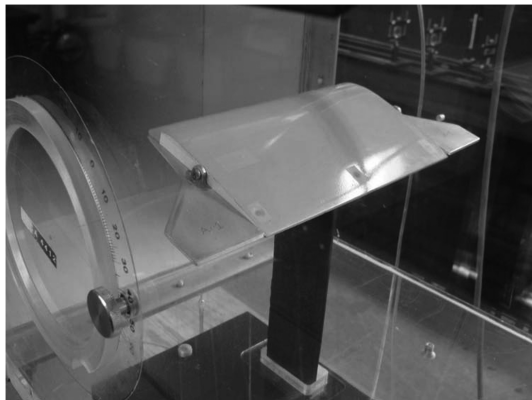
Fig. 5 Movable tip strakes MTS4A-1 installed on baseline wing in wind-tunnel test section.
