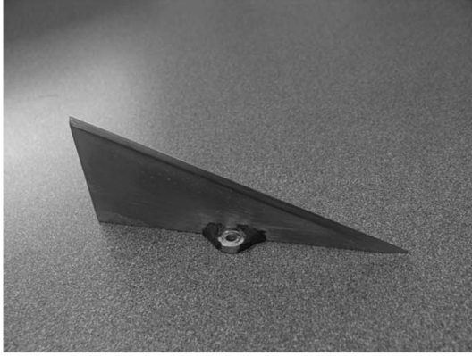
Fig. 1 Movable wing tip strake used to validate the concept.
